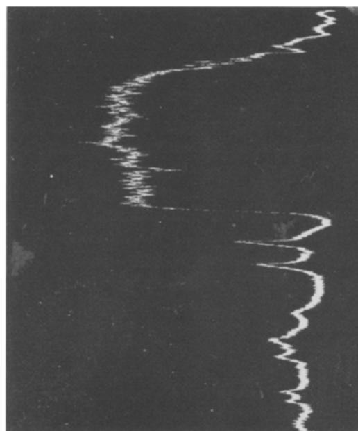
Fig. 6. X-ray image of \text{CoK}_\alpha (line analysis), magnification 1000\times and scanning electron microscope (SEM) image of Co-coating deposited on the hard metal under the same conditions as in Fig. 5a. Magnification 300\times .
